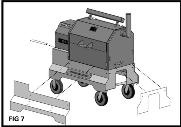
5. Install the back panel and hopper end panel by aligning the top edge of the magnet panel to the top edge of the comp cart. Starting from the top, smooth out the wrap to fit the contours of the panel and ensure all bolt holes line up. Center the hopper trim panel to the top side of the cart next to the hopper. If you are having issues with the back panel not fitting to the contour of the cart, try warming up the surface with a hair dryer as previously mentioned. (FIG 8)
